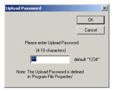
QuickControl will then ask for the password used for the file when it was downloaded. This is set in the Program File Properties dialog box (File ⇒ Program File Properties). The default is "1234".
