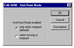
when moving or when holding position. This means that the servo can switch to open loop control whenever the position error is low enough, so an entire move could be executed using open loop control.
