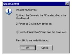
Verify your hardware is setup correctly (See Setup Start-Up Kit above). Do not connect the motor to a mechanical load until you are familiar with its operation and established any necessary safety interlocks. If your unit requires a clamp or clamp resistor, connect them now. Power up device and press OK.
