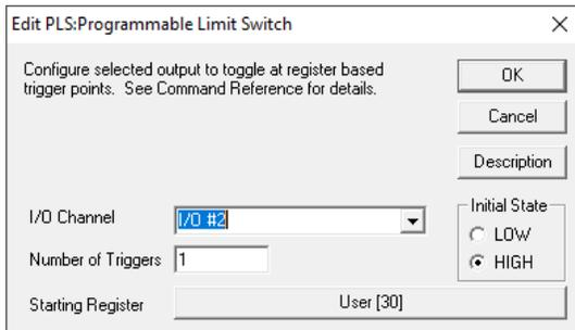
The programmable limit switch can be used to automatically toggle the selected I/O by comparing the position to one or more trigger registers, with the output toggling as each threshold position is passed. The I/O toggles back when the motion is in the opposite direction. See AN050 for more details.
