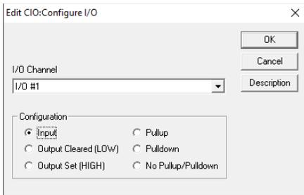
CIO x -1 (where x is 1 to 7) sets the main output to tristate for input mode.
