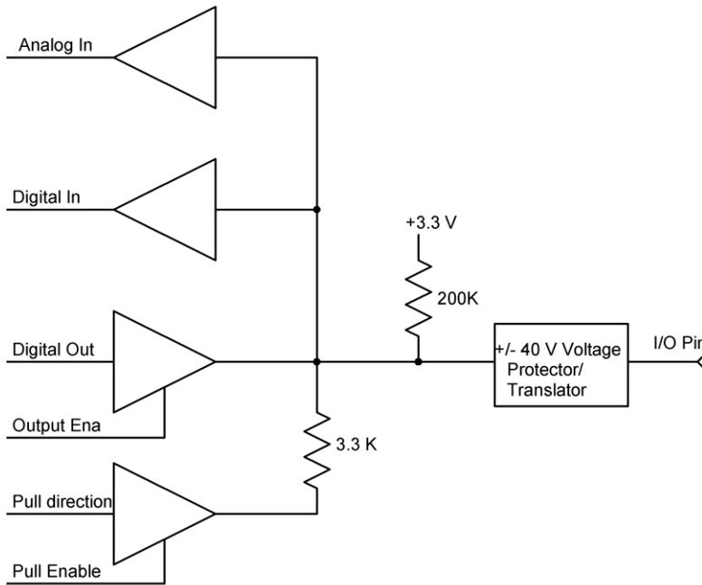
The top block in this figure is the analog input which can read the voltage present even when the digital portion is in operation. More accurate analog readings normally turn off the pull-up and driver signals. For details on using analog inputs, please see Application Note AN023.
