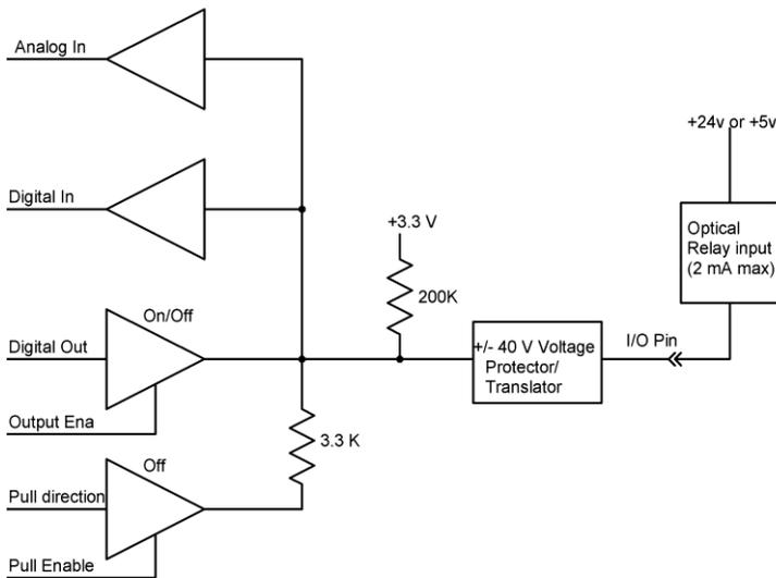
The output should be set to tri-state (input mode) so that the current on the internal side of the voltage protector drops to a low value so that the current at the output of the voltage protector will also be reduced to just leakage current.
