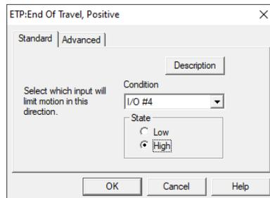
Any of the I/O can be used for end of travel limits, with either state being active. End of Travel Negative (ETN) sets the most negative limit, while End of Travel Positive (ETP) sets the most positive limit.
