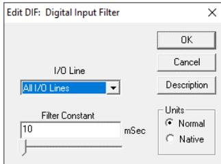
All the inputs are automatically filtered. The default is set in the initialization file, typically to 10 milliseconds to help eliminate issues with contact bounce. Each input can be separately configured to allow high speed registration to sample up to every 120µs without filtering. This filtering is not applied to PWM inputs, nor to encoder inputs which operate at much higher speeds.
