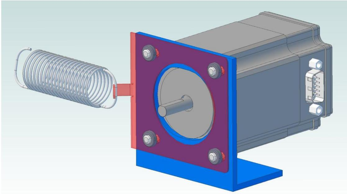
The drawing above shows the tensioning plate as semi-transparent only to allow the mounting plate behind it to be seen. This would normally be made of metal. The fish scale is shown as a spring; it is only present while setting the belt tension. After tightening the screws, the spring/scale is removed. A PDF version of this drawing is included which can be rotated for further information.
