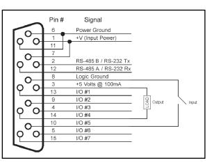
Note: Encoder Inputs on section 5 uses I/O # 4, 5, and 6 listed here. If these I/O are used for electronic gearing, they are **NOT** available for general purpose I/O function.
