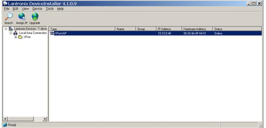
Select the wanted unit from the list. In this case, only a single unit is present. Click on the unit and then select "Assign IP". Select "Assign Specific IP address", NEXT
