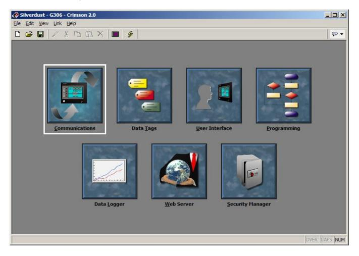
The program file, Silverdust.cd2, already has communications setup between the servo and the HMI for Unit ID 16, RS-232, and 57600 baud. This can be changed by pressing the Communications button.
